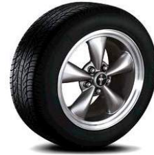
18" Premium Painted Cast Aluminum Wheel w/Machined Outer Lip, Small Tri-bar Pony Center Cap Std. on Bullitt™ Pkg. only {140A} (54B)
